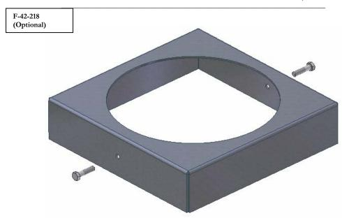
FP-42 FLUE TO HT CHIMNEY ADAPTER, F-42-218
